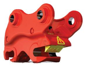
The PowerLatch™ has a secondary mechanical backup system in place that is completely independent of the hydraulic circuit which locks on both the front and rear attachments pins to ensure that they remain securely attached in the event of a loss of hydraulic pressure.
